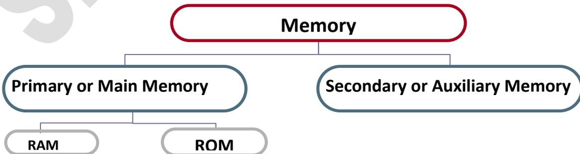
**Main Memory / Primary Memory:** - Memory which is directly connected to the CPU is known as Main Memory or Primary memory. It is also known as short-term memory. There are two types of Main Memory.
